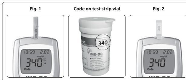
**Coding is only possible if the measurement device is turned off!**
